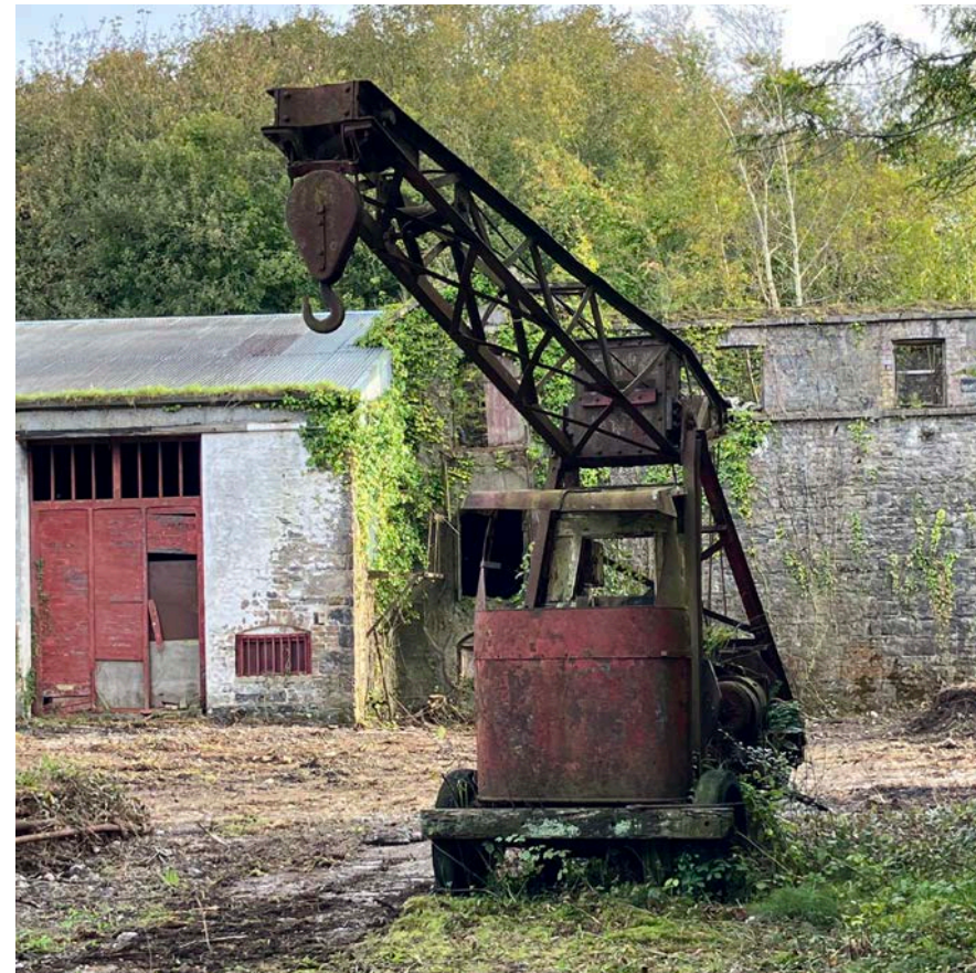
Figure 91 - Crane - Three and a half ton mobile crane
